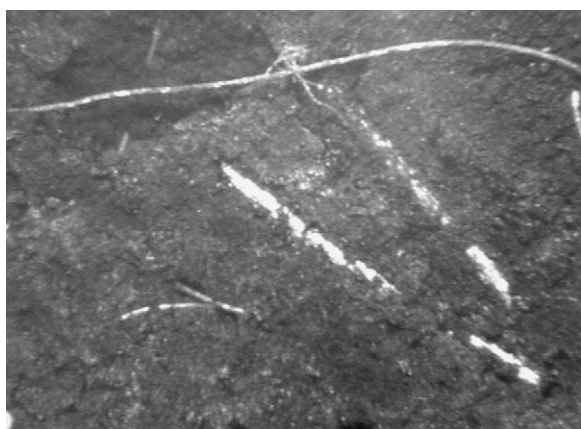
Fig. 5. Ti wire (76 μm dia.) in positive paste taken after cycling tests. Optical microscope at 4× magnification.
